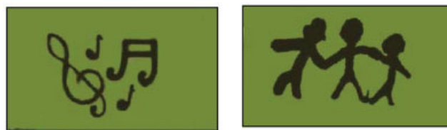
Figure 9 Image recording of P-10 by UV irradiation through masks; a black background was set behind the polymer film.
